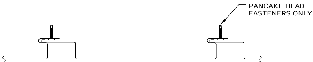
FW SERIES CUSTOM REVEAL SEAM ENGAGEMENT
