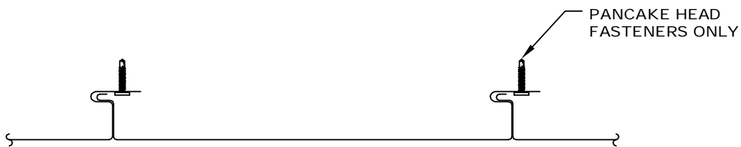
FW SERIES TYPICAL SEAM ENGAGEMENT
