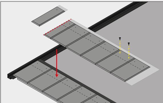
READYSLATE® slate tiles are marked with an overlapping line to ensure all modules are easily and correctly laid.
