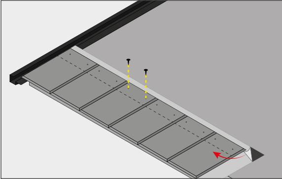
READYSLATE® is easily installed with nails. All individual slate tiles are predrilled to simplify the installation process. Once fitted, peel back the protective film.
