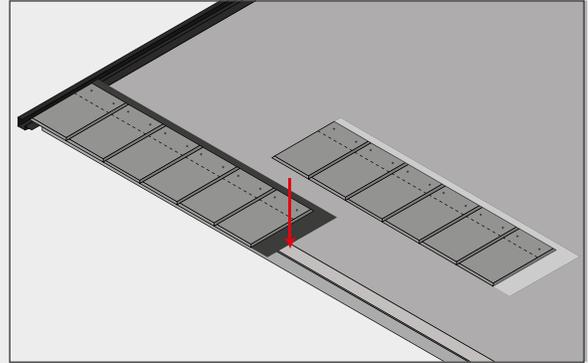
READYSLATE® modular design makes laying slate tiles a breeze. Aligning modules is even easier; just cover the spare area on the waterproof sheet.
