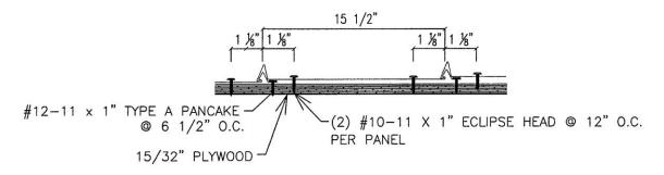
Figure 1. 1.5" Nailstrip Panel Detail (Minimum 24 Gauge)
